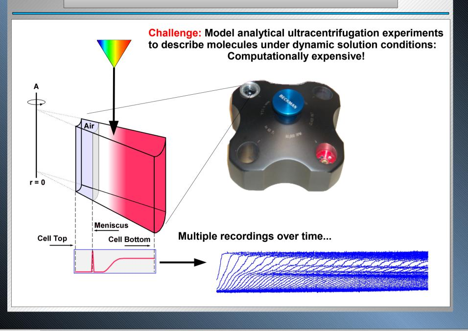
$$L(s,D): \left(\frac{\partial C}{\partial t}\right)_{r} = \frac{-1}{r} \frac{\partial}{\partial r} \left[s \omega^{2} r^{2} C - D r \frac{\partial C}{\partial r}\right]_{t}$$
